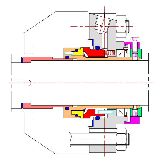
90 SERIES MULTI SPRINGS BALANCED SLURRY MECHANICAL SEAL TYPE 9602 CARTRIDGE ARRANGEMENT WITH DIFFERENT API PLAN 62
